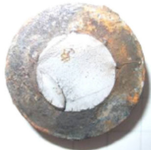
Fig. 11. View of the shank section of one failed rivet.
