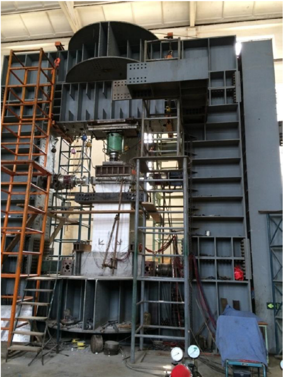
Pseudo-dynamic test setup (Information provided by C.A.B.R. China Academy of Building Research, 2014)
